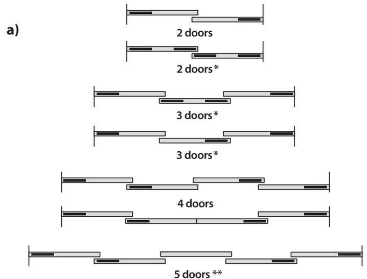
\* In 2-door or 3-door arrangements where two soft-closers are fitted to each end of a single door, the door must be a minimum width of 850mm to allow both soft-closers to be installed. Doors fitted with a single soft-closer must be a minimum width of 500mm.
