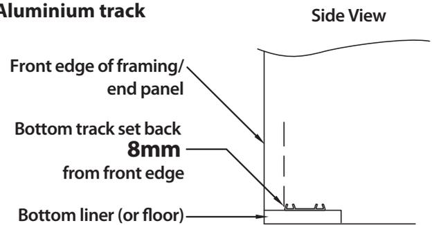
**IMPORTANT** - Please slide door positioners into the aluminium bottom track before fixing to the floor liner (see illustration **c**). Door positioners are not required for a two door system if the bottom track is level. Refer to section **8.2** for final positioning.
