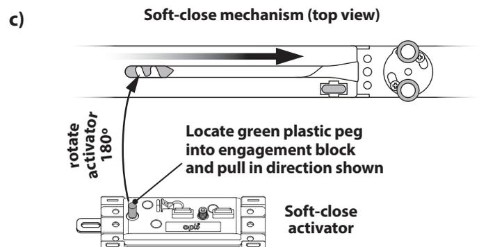
Depending on whether you have ordered aluminium- or steel-framed doors follow the appropriate instructions below for fitting the soft-close activators:
