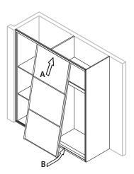
Repeat the process with the front door(s), using the front channel and front bottom track. For multi door systems alternate the doors on the tracks.
